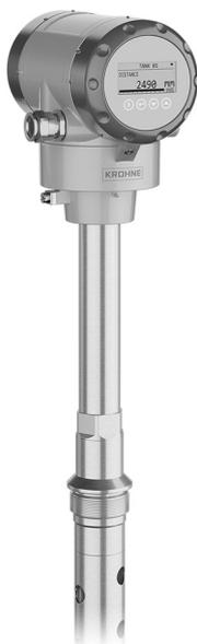
The OPTIFLEX 7200 is designed specifically for measuring level and interface in the chemical, oil and gas industries. It can be used in high tanks (max. height 60 m / 197 ft) and pressure vessels.
