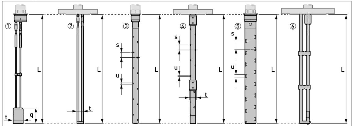
Figure 2-22: Double probes and coaxial probes: options and overall dimensions
