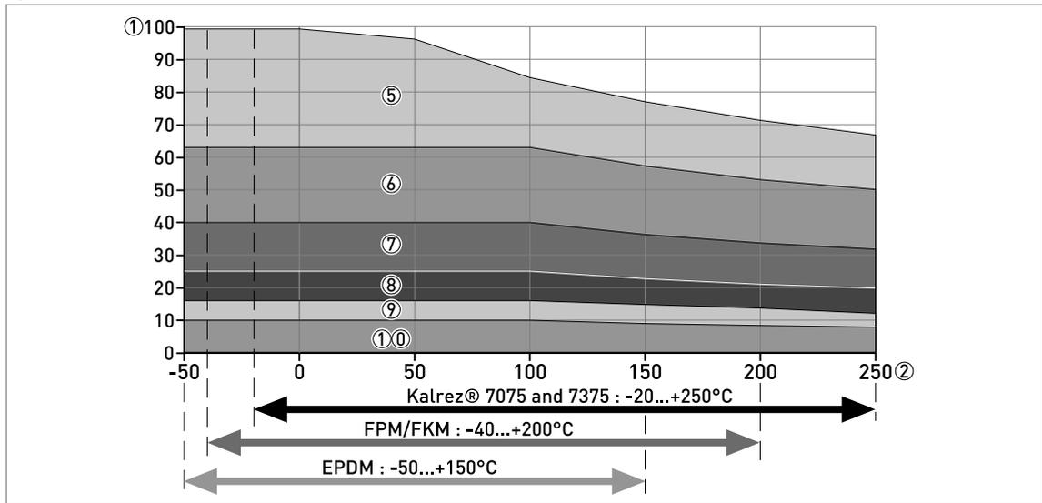
Figure 2-5: Operating limits for devices with single ceramic process seal system: graph of process pressure (barg) against process connection temperature (°C)
