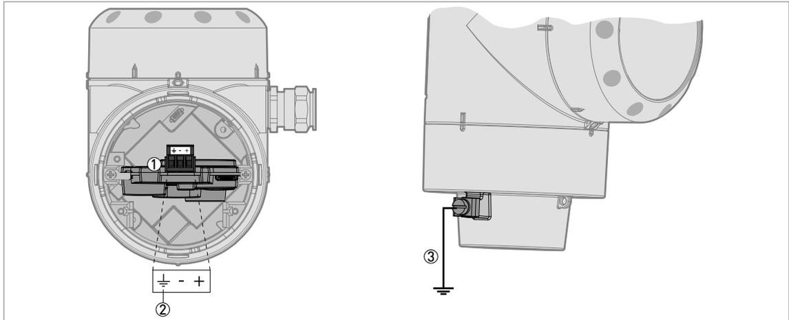
Figure 4-1: Terminals for electrical installation (one output)
