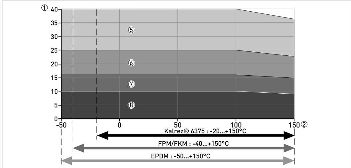
Figure 2-3: Operating limits for devices with a single PTFE process seal system: graph of process pressure (barg) against process connection temperature (°C)
