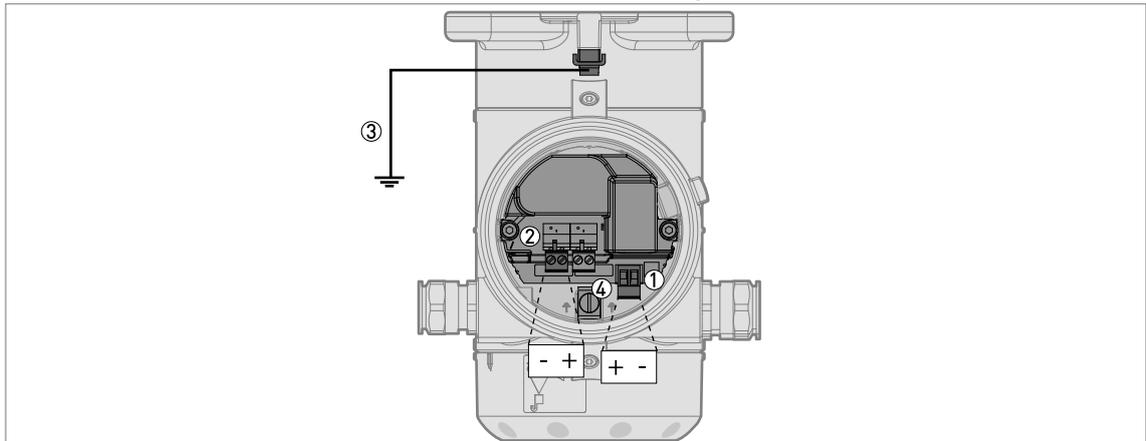
Figure 4-5: Terminals for electrical installation (two current outputs)
