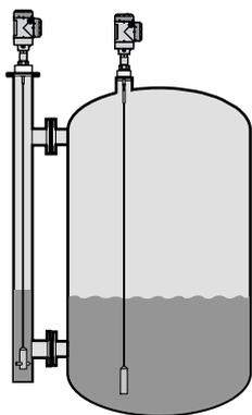
The level transmitter can measure the level of a wide range of liquid products on a large variety of installations within the stated pressure and temperature range. It does not require any calibration: it is only necessary to adapt the probe length and do a short configuration procedure.
