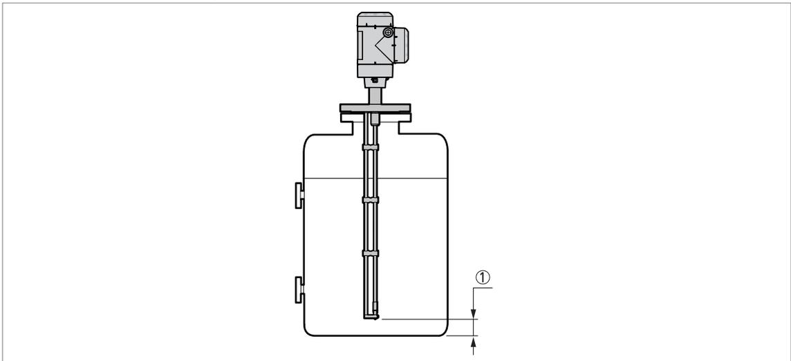
Figure 3-6: Minimum limits for the installation of the reversed interface probe
