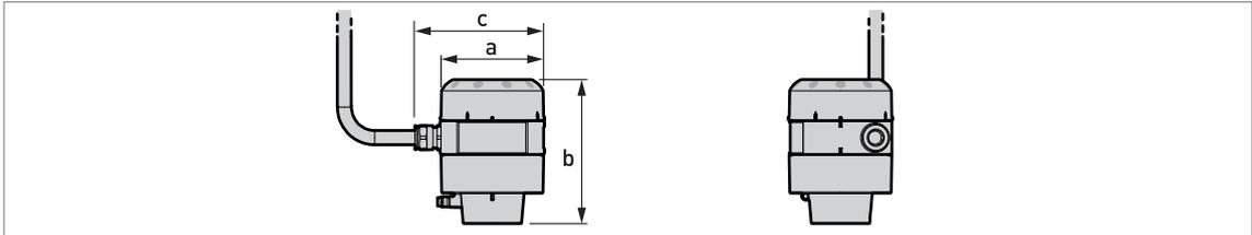
Figure 2-17: Remote version (F) – probe electronics housing
