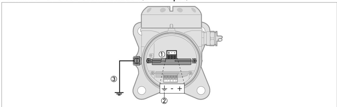
Figure 4-4: Terminals for electrical installation (one output)
