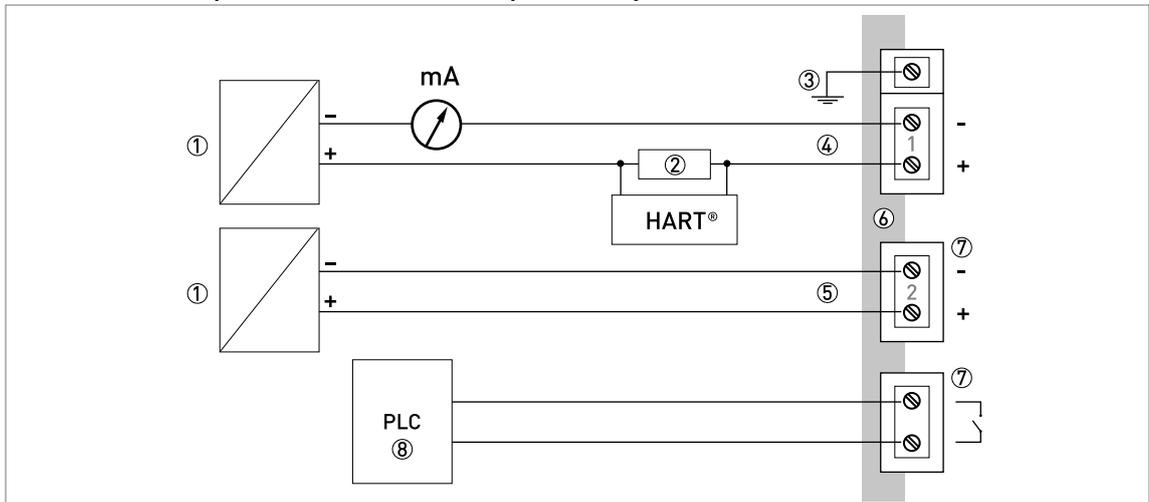
Figure 4-10: Electrical connections for non-Ex devices (one current output and one switch output - relay)
