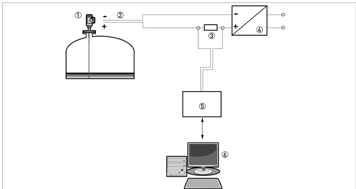
Figure 4-11: Point-to-point connection
