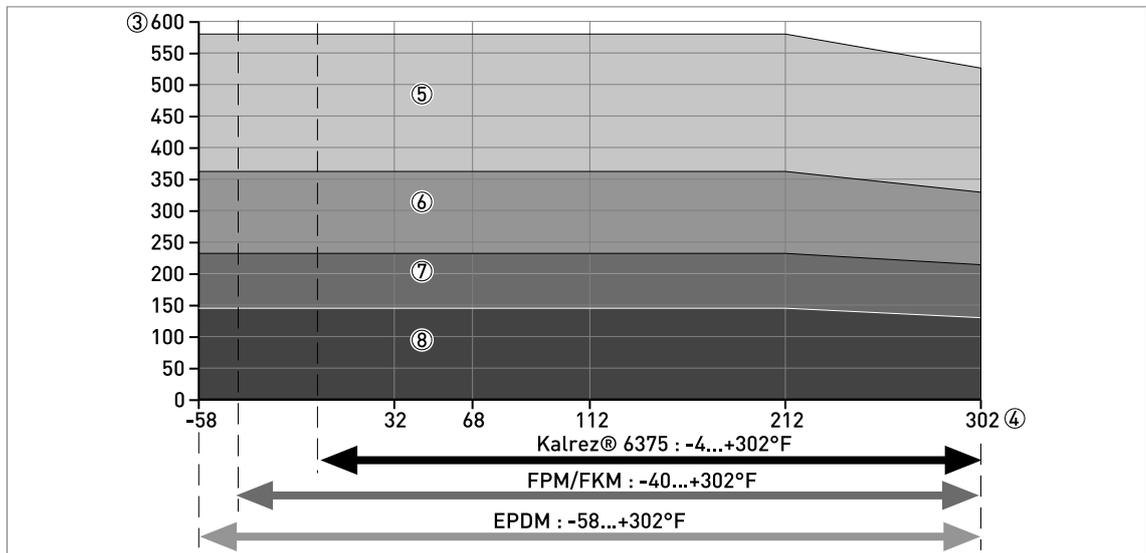
Figure 2-4: Operating limits for devices with a single PTFE process seal system: graph of process pressure (psig) against process connection temperature (°F)
