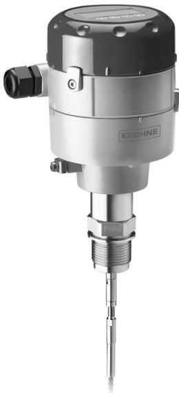
OPTIFLEX 1100 C is a 2-wire TDR level transmitter for measuring distance, level, volume and mass of liquids and solids. Its simple, compact design allows technicians to quickly assemble the probe and attach it to a threaded connection. It is an affordable solution for applications that do not require a high level of accuracy and is also an excellent alternative to traditional level controls such as RF Capacitance, conductive and DP transmitters.
