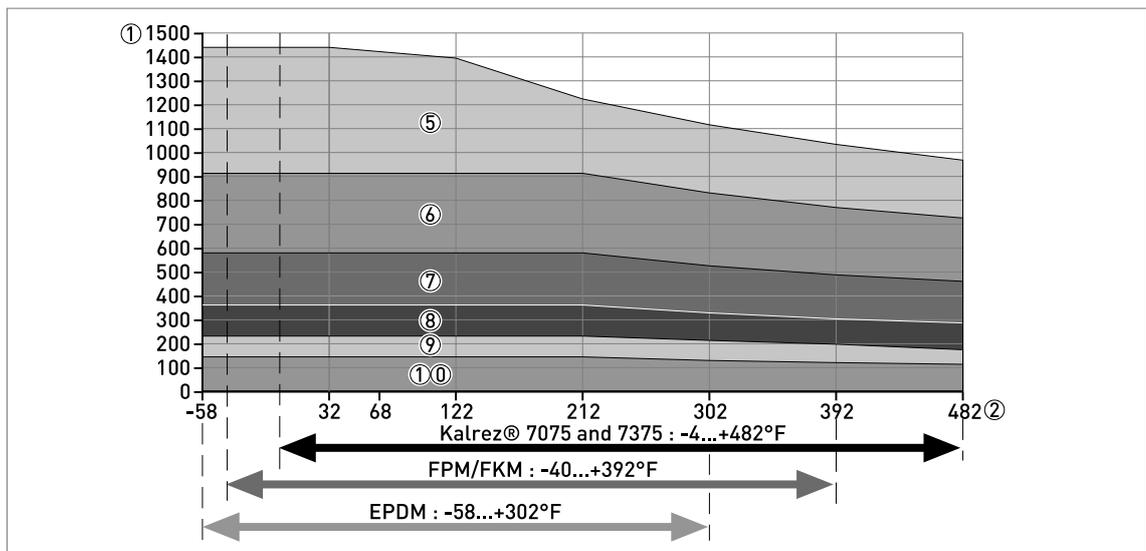
Figure 2-6: Operating limits for devices with a single ceramic process seal system: graph of process pressure (psig) against process connection temperature (°F)
