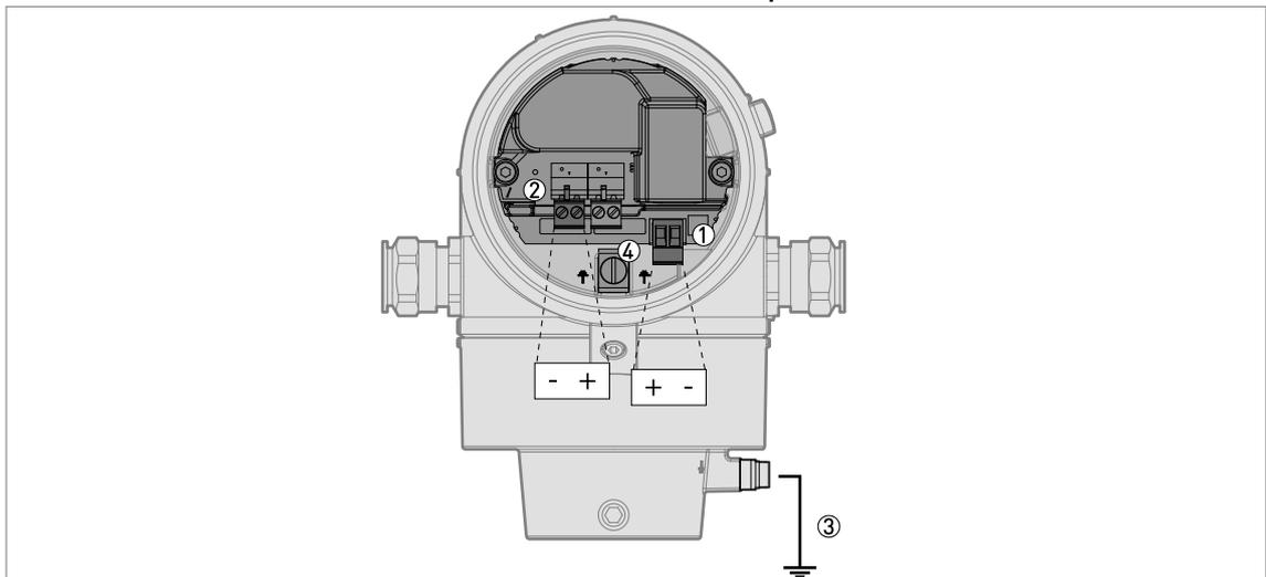
Figure 4-2: Terminals for electrical installation (two current outputs)
