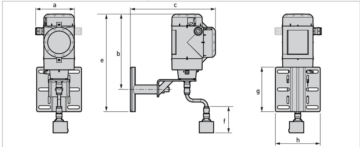
Figure 2-13: Sensor extension with vertical compact version (S)
