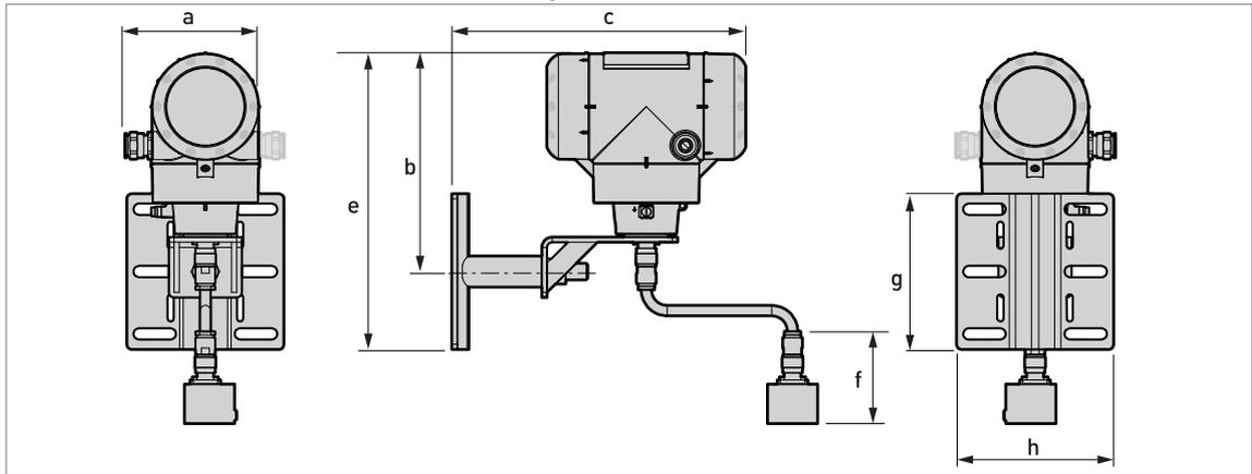
Figure 2-14: Sensor extension with horizontal compact version (S)
